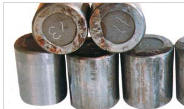
Part: Tapered rollers of a double-row tapered roller bearing Symptom: Stepped wear on the roller end face Cause: Fretting progression due to excessive load while stationary
