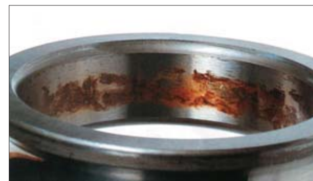
Part: Inner ring of a deep groove ball bearing Symptom: Fretting occurs on the bore surface Cause: Vibration
