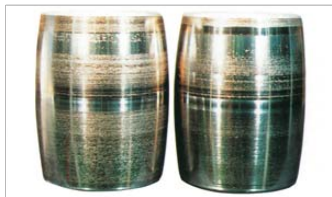
Part: Convex rollers of a spherical roller bearing Symptom: Smearing occurs at the center of the rolling surface Cause: Incorrect lubrication
