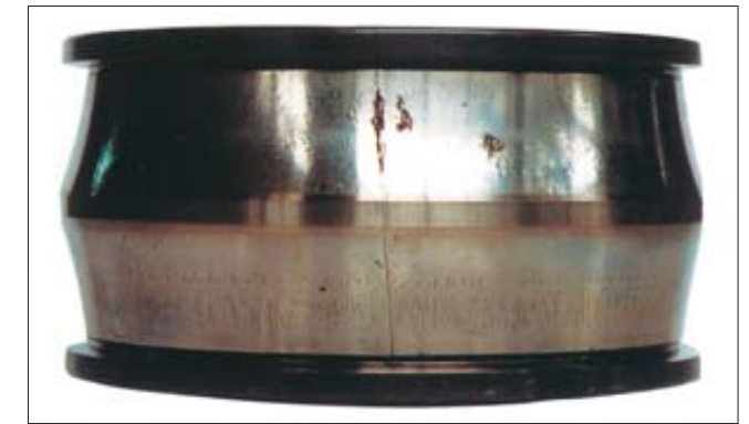
Part: Inner ring of a spherical roller bearing Symptom: Axial cracks occur on raceway surface Cause: Large fitting stress due to temperature difference between shaft and inner ring
