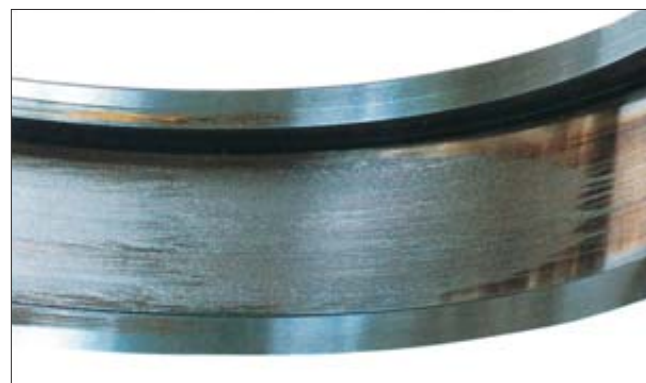
Part: Outer ring of a cylindrical roller bearing Symptom: Smearing occurs circumferentially on raceway surface Cause: Roller slipping due to excessive grease filling
