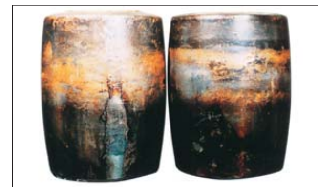
Part: Convex rollers of a spherical roller bearing Symptom: Discoloration and melting of roller rolling surface, adhesion of abrasion fragments from cage Cause: Insufficient lubrication
